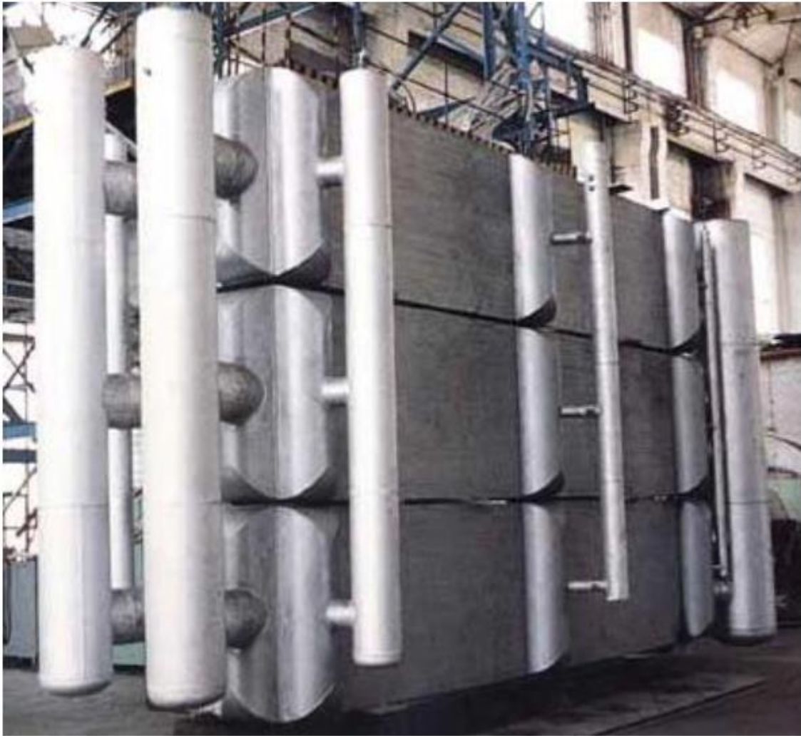
Figure Error! No text of specified style in document..103: Plate fin heat exchangers typically made of aluminum and brazed together Source: http://webwormcpt.blogspot.com/2010_07_01_archive.html (typically used for cryogenic service)
