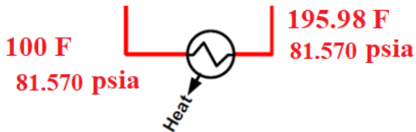
Figure Error! No text of specified style in document..77: Aftercooler downstream of compressor 2
